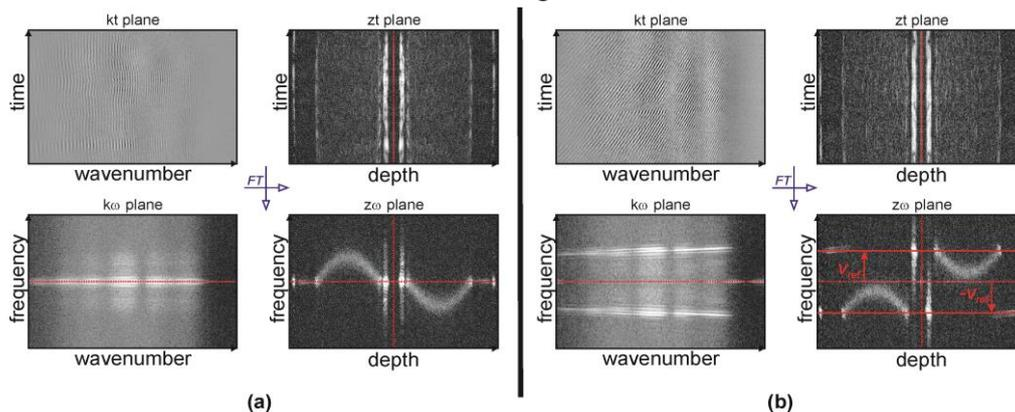
Fig. 5. STdOCT diagrams of scattering fluid flow in a glass capillary. (a) data collected in a standard configuration with a fixed reference mirror; (b) with an additional velocity  $v_{ref}$  set by the mirror in the reference arm. Additional velocity causes movement of the image and its complex conjugate in opposite directions along the axis of frequency and allows them to be easily separated, even if the images overlap along the depth axis. Figure is taken from [IB.3].
