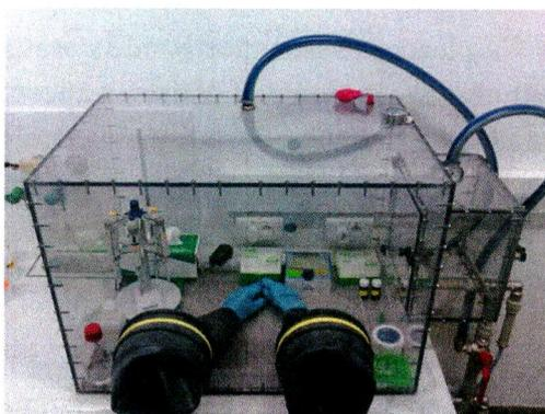
Fig. 5 Handmade glovebox from my project at NCU.
